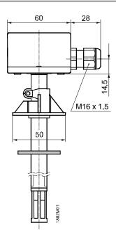
Drilling template with (without) mounting flange
