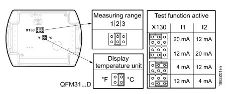
The setting elements are located inside the cover. A setting element consists of 6 pins and a jumper. It is used for selecting the required temperature measuring range and for activating the test function. Types with LCD display have a second setting element with 4 pins and a jumper.
