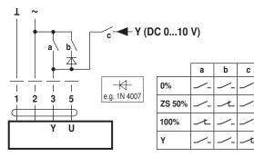
Control remotely 0...100% with Minimum limit with positioner SG..
