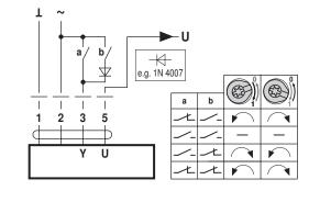
Control with 4...20 mA via external resistor
