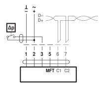
Modbus RTU / BACnet MS/TP with analogue setpoint (hybrid mode)
