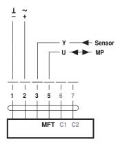
Requirements for switching contact: The switching contact must be able to accurately switch a current of 16 mA @ 24 V.
