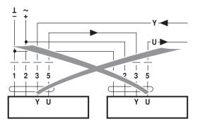
Control with 4...20 mA via external resistor
