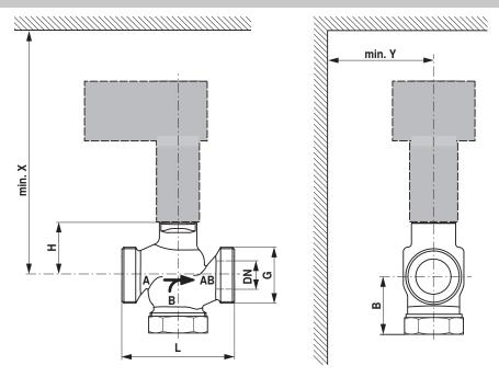
X/Y: Minimum distance with respect to the valve centre. The actuator dimensions can be found on the respective actuator data sheet.
